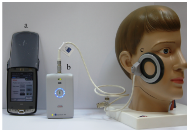
Fig. 2 The energy delivery control subsystem (EDC). The three parts of the EDC are shown: (a) controller; (b) driver; (c) transmitter.
